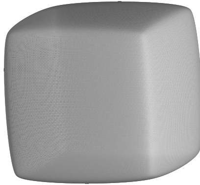
Figure 5: Wulff shape W_\gamma for regularized l^1 -anisotropy, with W_\gamma = \{\mathbf{z} \in \mathbb{R}^3 \mid \mathbf{z} \cdot \mathbf{q} \leq \gamma(\mathbf{z}) \, \forall \mathbf{q} \in \mathbb{R}^3\} .
